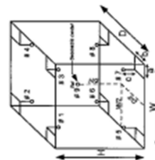
Figure: Example of sensor installation locations
